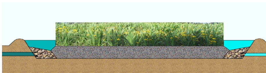
Figure 4: Surface flow constructed wetland
